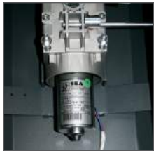
Electric motor with low absorption Motor a baja absorción
