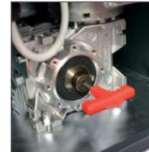
Release with personalized key Desbloqueo manual
