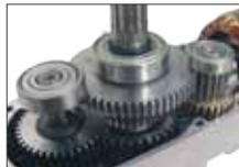
Thermo treated gears on rotating arms supported by ball bearings
